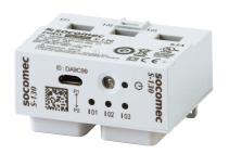
DIRIS Digiware S current measurement modules have 3 integrated current sensors for measuring, monitoring and analyzing power quality of electrical circuits up to 63 A.
