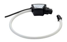
TF flexible Rogowski coil current sensors are used with DIRIS Digiware I, DIRIS A, or DIRIS B Power Monitoring Devices to measure currents from 100 to 6000 A with the same guaranteed accuracy. The quick RJ12 connection, and the integrated intelligence prevent any connection or configuration errors.
