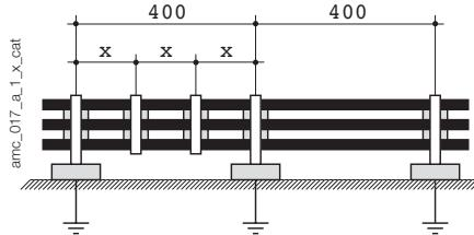
Flexible bars should be mounted on insulated supports with a maximum distance of 400 mm. Bars should also be held together with straps, as shown in the above diagram. The distance between successive straps depends on the electro-dynamic constraints in the event of a short-circuit. The table below gives the recommended distances between straps.
