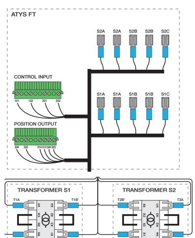
These Faston are to be connected in the switching mechanism on source 1 and source 2 poles under the power connectors as shown below.
