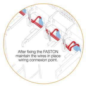
The wires should be passed along the cable duct as shown below (this includes cables with unused Faston connectors).
