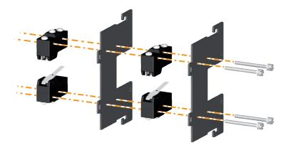
Then fix the assembled products on the switch:
