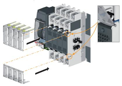
When fixing the shrouds make sure the pieces fit in the switch as shown in the image above then push back to clip in place.
