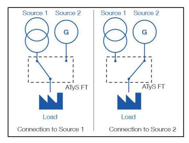
These automatic transfer switches are designed to meet NFPA 110 requirements for NFPA 110 for Emergency and Standby Power systems and the National Electrical Code (NEC) Articles 700, 701 and 702.
