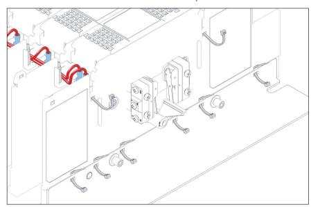
For example, these can be used to maintain cables in place when connecting wires to the customer position auxiliary contacts.
