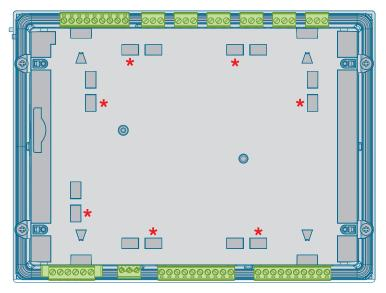
Cable ties used should be adapted according to the position of the door:
