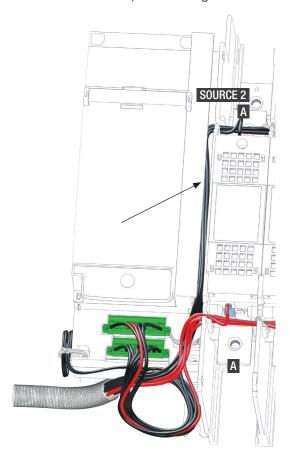
Pull the cables down so that all wires are tight and use a cable tie to maintain all cables coming from the cable duct into place (cf. image below):
