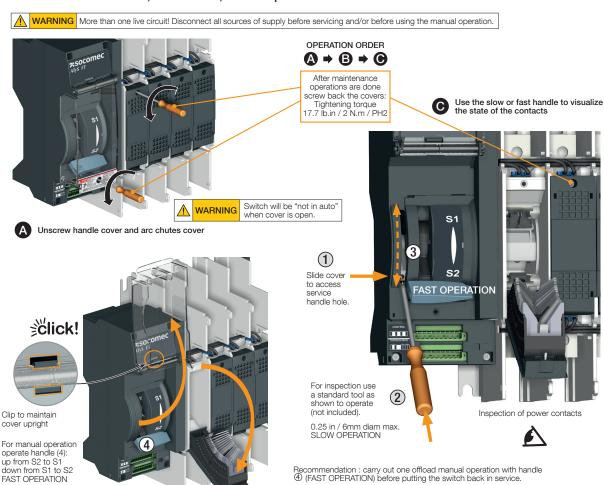
Reverse the procedure to close. Ensure that all is closed properly before putting back in service. In case any part of the ATyS FT switch is found to be damaged in any way, replace the complete switch.
