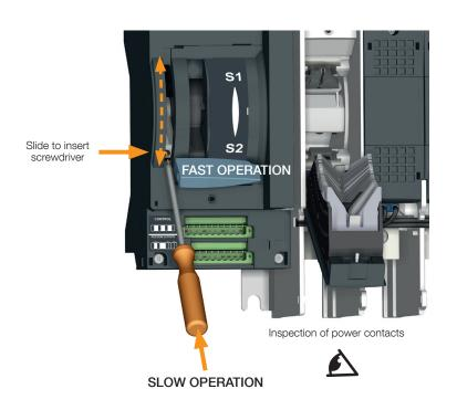
CAUTION! Once all manual operations are completed make sure to screw back the arc chutes and plastic protection cover in place, tightening torque 17.7 Lb.in (2 N.m) using PH2 type screwdriver.
