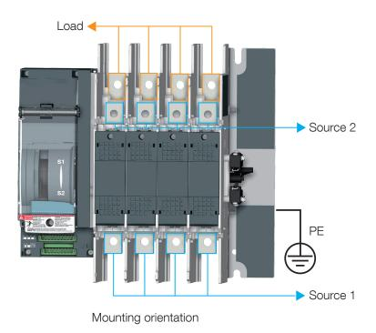
Socomec recommends connecting the Emergency (or alternate) source on the Source 2 power connections and the Normal (primary) source on the Source 1 power connectors.
