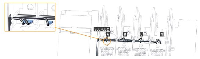
The Faston connectors must be placed specifically to match your network, in order to do this refer to the tables below: For harness without transformer:
