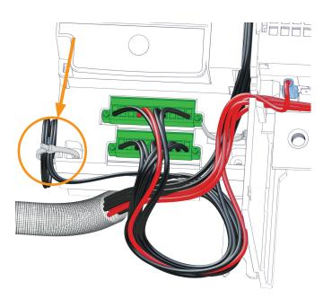
This switch includes additional cable tie fixation points as show in the following image.
