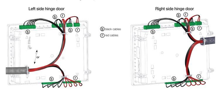
CAUTION! Cables must be more than 0.4 in (10mm) away from the RTC battery cover and USB connector.
