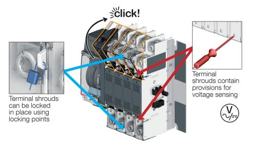
Terminal shrouds can also be fixed in place using cable ties as shown below, they also include small diameter holes to allow for voltage sensing without removing the covers.
