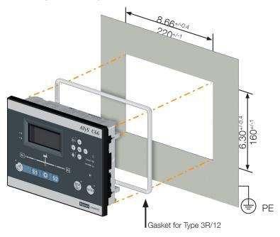
For NEMA 3R12 protection the gasket must be placed and fitted on the inside perimeter of the controller.
