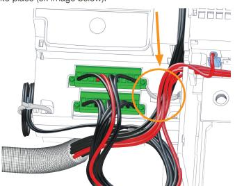
Then fix any cables with unused faston connectors on the side of the switch as shown below:
