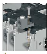
Mount the load terminal lugs on the switch terminals before mounting source 2 terminal lugs.
