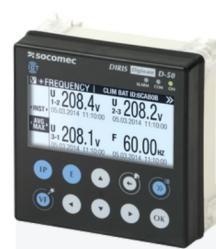
The DIRIS Digiware D-50 and D-70 are panel mount displays for local visualization of measurements from the entire DIRIS Digiware SBCM system. They also act as communication gateways, communicating measurements via RS485 or Ethernet (Modbus RTU, Modbus TCP/IP, SNMP, BACnet IP). With the DIRIS Digiware D-70 display, measurements can be visualized on WEBVIEW-M, a web-based energy management software embedded in the D-70 display.
