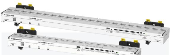
The DIRIS Digiware BCM is a branch-circuit monitoring strip with 21 integrated current sensors for the individual circuit monitoring within Remote Power Panels (RPPs) or electrical panel boards.
