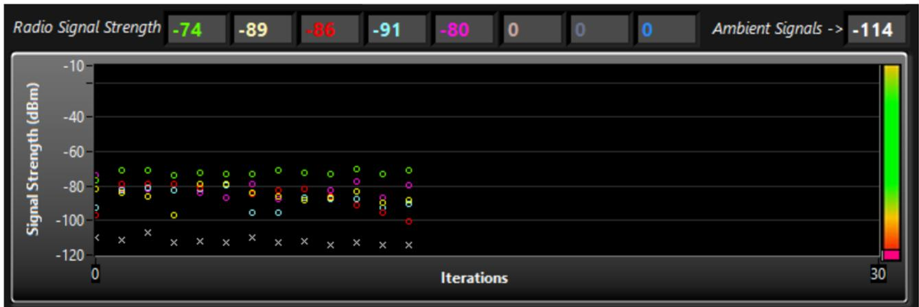
The signal strength is also charted for each received radio response and reported in the units of dBm ranging from -10 to -120. A color chart is provided at the right-hand side of the plot. Normal signal strengths are in the -60 to -95 range for typical application. The ultimate limit of communication for this system is -108 db although the error rate will be unacceptable at this low signal level.
