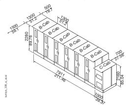
**Back-to-back installation (with 1 C-Cab)** Up to 6 B-Cabs - dimensions (mm/in)
