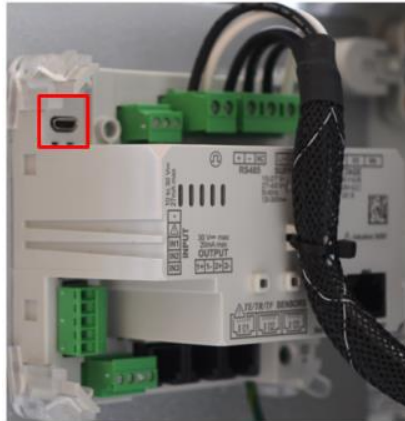
Figure 8: The micro USB port on the DIRIS A-40
