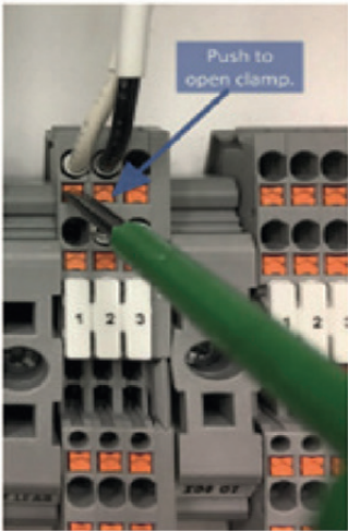
Figure 131. Operating C-Cab XXL Terminal Blocks
