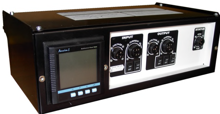
Figure 1-1: SMART-R2B shown with External Measurement Port (EMP) option (cover removed)
