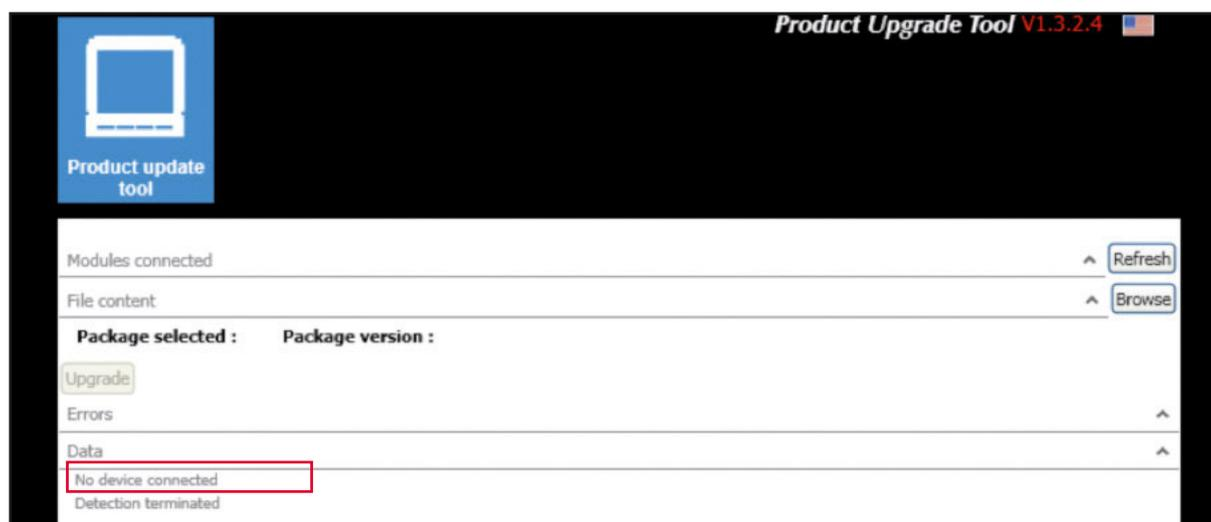
If the module is not recognized, change the USB port and click “refresh” or check if the module is supplied
