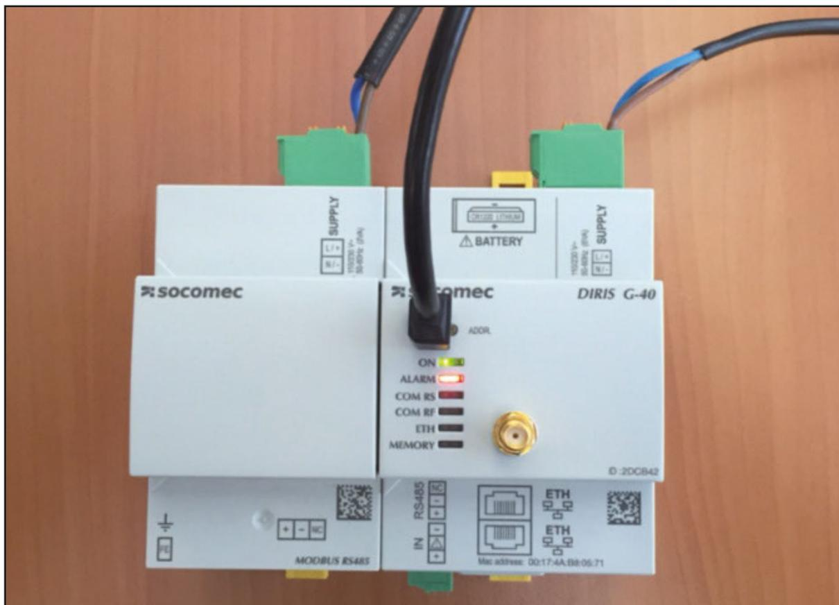
We will carry out an upgrade of the versions 1.3.0.11 (G-40) to the 1.4.9 version for the G-40 gateway and a downgrade of the 1.3.0.2 version 1.2.0.19 version for the Com module:
