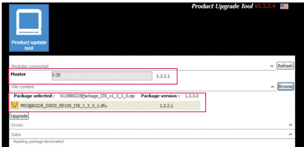
Note: When the package is loaded, you can see on the screen the information of each firmware that is going to be updated.
